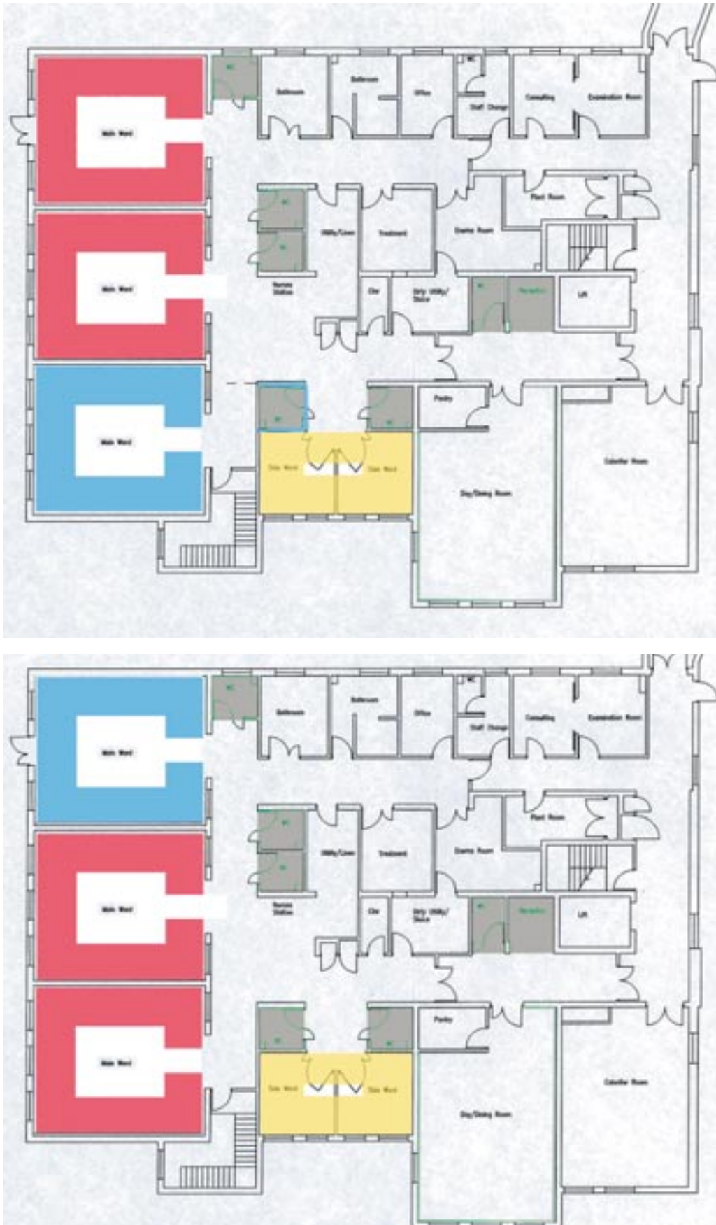
Figure 10. L-shaped wards: this plan can work with a 2/1 bay mix providing the two same sex bays are adjacent, but fails if the bays are split. The two single rooms are flexible in use. It may be possible to modify the layout of one WC to provide en-suite facilities to one six-bed bay. An additional toilet opposite the day space (outlined in green) would be beneficial
