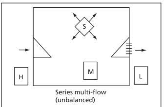
**A8.21** Where the room has a net surplus of mechanical supply air, a transfer grille should be located in or adjacent to the door through which air flows outwards, and the mechanical supply flow rate to the room should be chosen to give protection when this door is open.
