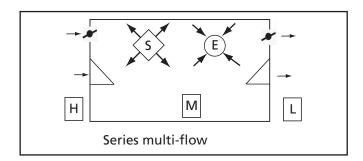
**A8.25** These transfer devices will normally be pressure stabilisers, although transfer grilles may be used where a large amount of excess air is to be exhausted from the operating theatre when all doors are closed (for example anaesthetic rooms).
