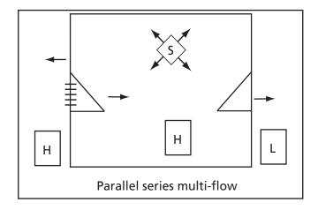
**A8.18** Where the nominal room pressure equals that of the higher-pressure adjacent room, the best use of air is by supplying air required for bacterial dilution only and allowing this to exhaust via a transfer grille to the area of equal cleanliness. The doorway to the lower pressure area is protected by the combination of the supply air and the air that will flow inwards through the transfer grille from the area of equal cleanliness.
