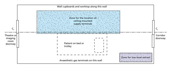
The above shows the typical zones for the positioning of ceiling-mounted supply and low-level extracts in an anaesthetic room. The objective is to comply with the COSHH Regulations and HTM 03-01 Part A by providing a clean airflow path for staff working in anaesthetic rooms and so reduce their risk of casual exposure to waste/leaking anaesthetic agents.
