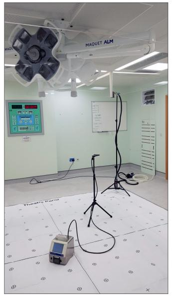
**12.96** The detector will be an LSAPC capable of sampling a minimum of 28.3 L of air (1 ft<sup>3</sup>) per minute and providing readings for particle sizes from to 5  $\mu$ m to 0.3  $\mu$ m. The instrument should be compliant with the requirements of BS EN ISO 14644. An alternative instrument may be used providing it is of no lesser specification.
