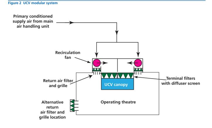
having a slightly different approach to UCV design. Whichever system is used, in order for the UCV terminal to produce the desired airflow within its footprint without entraining non-filtered air, the physical outside edge of the UCV canopy unit should not be less than 1 m from the operating theatre wall.
