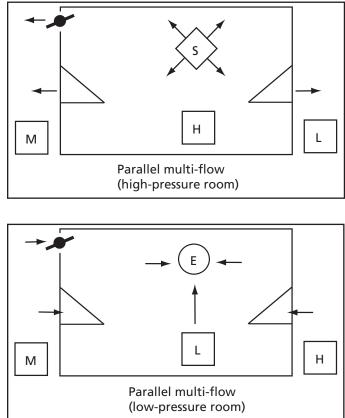
**A8.15** These rooms will be either highpressure or low-pressure with respect to the adjacent areas (see preparation lay-up room and disposal room, respectively, in standard layout 5 of Appendix 7). The pressure-relief damper is always situated between the room and area, which results in the smaller differential pressure to ensure best use of air.
