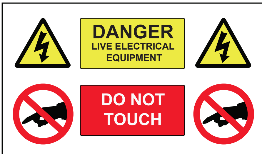
Figure 5 Danger sign (actual size: 200 x 100 x 1.5 mm white plastic)
