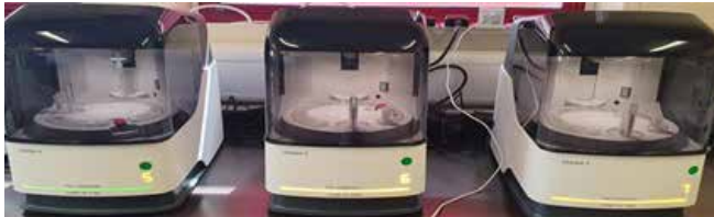
Three of our SAMBA machines processing patient samples to test for COVID-19
