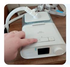
If your CPAP machine does not start blowing air, press the 'on' button to turn it on.
