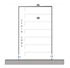
This shows an existing building with more than 2 residential units on level 3B. The building is 7 storeys high. 3B has no separate entrance from and exit to the outside so it cannot be an "independent section", and so the whole building has to be registered with the BSR as one building.
