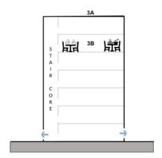
3A is a 7-storey hospital, so is an HRB. It has a cafe on level 3B. The cafe has no separate entrance from and exit to the outside so it cannot be an "independent section" for building works.
